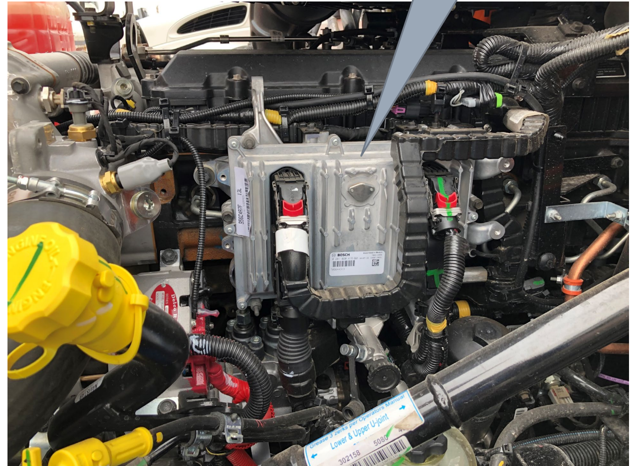
The driver's side of a Navistar A26 Engine in an International LT truck.
