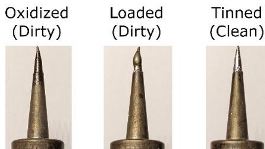
Figure 19: Three stages of cleaning a soldering iron tip.
