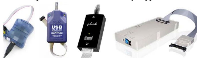
Figure 31: Examples of microcontroller specific debuggers and programmers: AVRISP mkII, Multilink, J-Link, TRACE32
