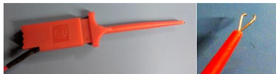
Figure 25: Close up of a mini grabber test clip (left); detail of open mini grabber claw (right)
